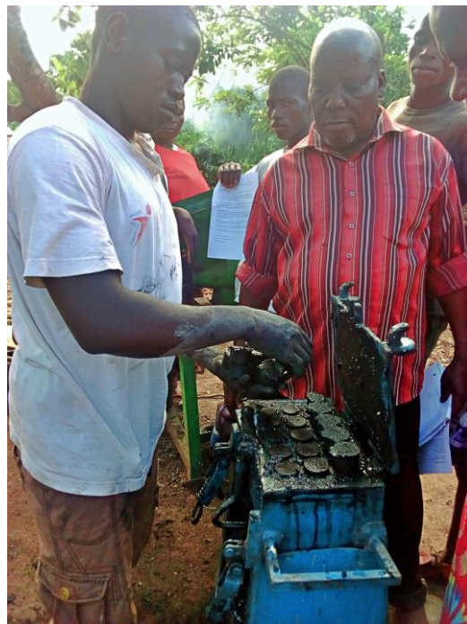
One special feature of this seminar was training in how to make fuel briquettes from waste materials
