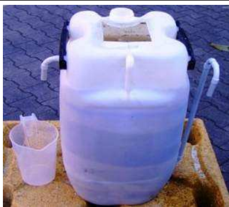
A home-made water filter in Germany which shows both types of outlet pipe
